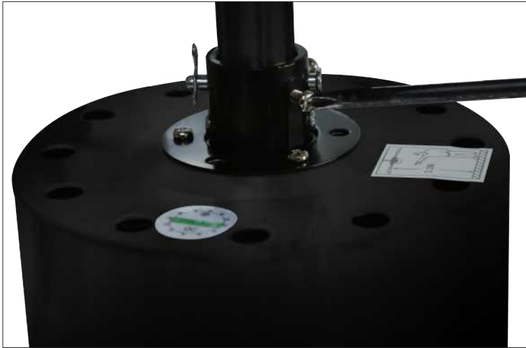
Step 8 Tighten the 2 screws of the coupler.
