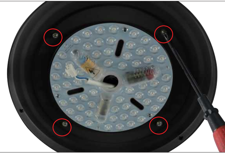
Step 18 Fix the light kit with the screws.
