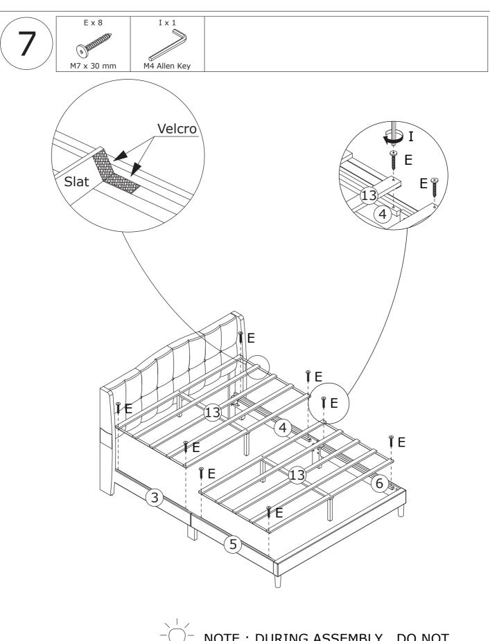
NOTE: DURING ASSEMBLY, DO NOT TIGHTEN ANY SCREWS UNTIL THE COMPLETE UNIT HAS BEEN ASSEMBLED.
