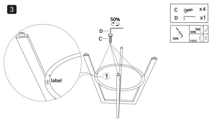
Remark: When installing the footrest, note that the side with the label ① is installed facing up.
