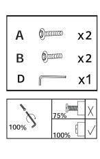
Remark: Install the 2 Bolts B on the holes near the backrest side. Screw the 2 Bolts A into the holes near the cushion side.
