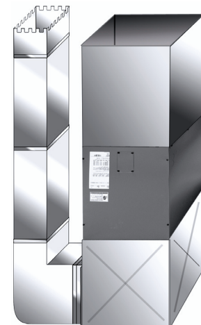
Assembled system features the Return Air Box (RAB), used with the Plenum (WKDP), Air Handler (WMA), and the Return Air Drop (RA 16).
