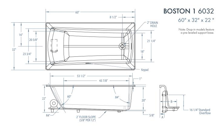
FEATURES Dimensional Tolerance ± 38". Dimensions needed for site preparation should be measured from the unit. Manufacturer assumes no responsibility for preparatory work.
