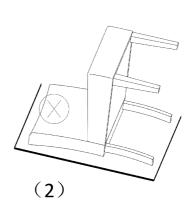
Place the chair onto the side of a table as seen in picture 1. Position Front Leg(C) into Chair Seat(B) and attach using Bolts(②), Spring Washers(②) and Washers(②) with Allen Key(③). Repeat same step to attach Right Front Leg (C) to Chair Seat(B).
