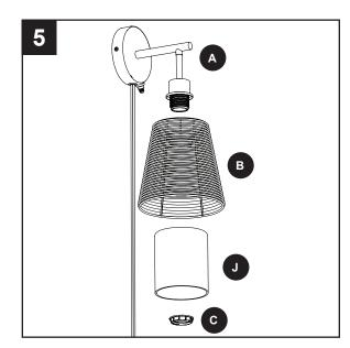
6. Install medium-base (E26) bulb (sold separately) in socket of fixture (A).
