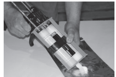
FIGURE 13: LEVELING THE PLUNGERS
