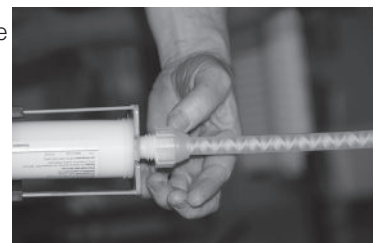
FIGURE 14: ATTACH STATIC MIXING TIP
