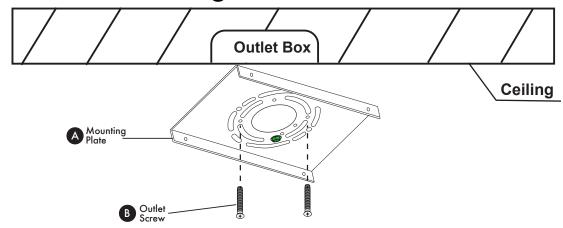
Align mounting plate (A) and outlet screws (B) with outlet box.
