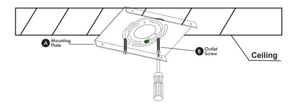
Attach mounting plate (A) to outlet box with outlet screws (B). Secure with Phillips head screwdriver or drill.
