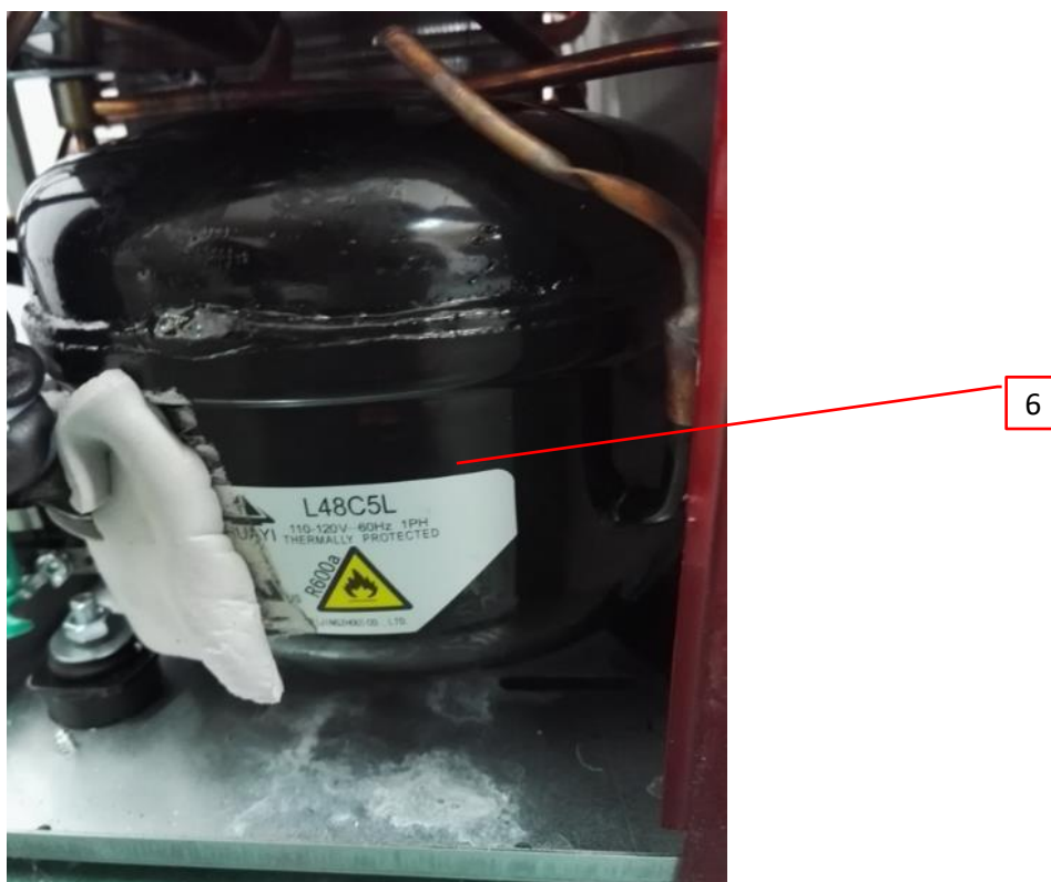
Photo 16 - Local construction of compressor L48C5L - HZB-12/B
