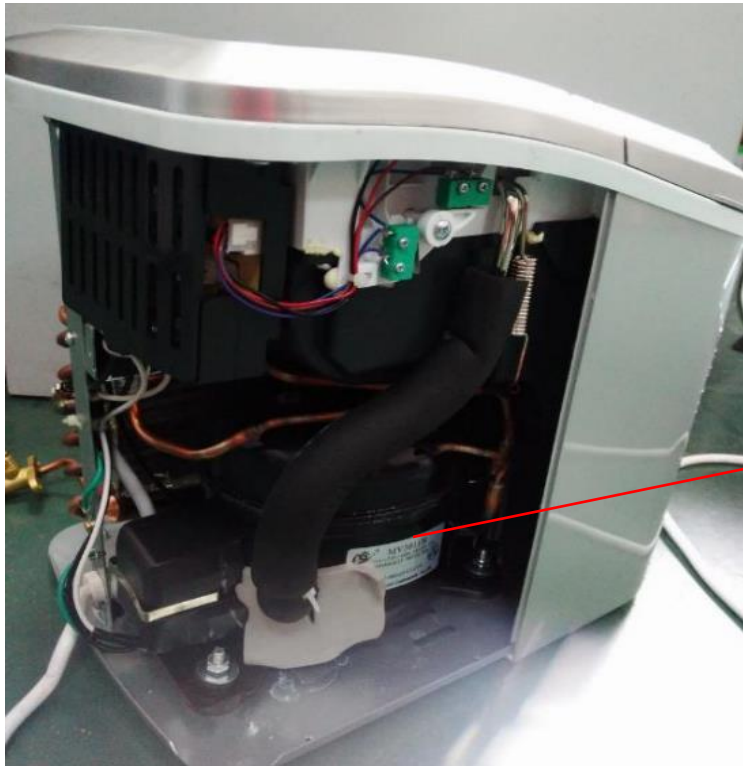
Photo 13 - Alternative compressor MV3011H manufactured by Liyang
