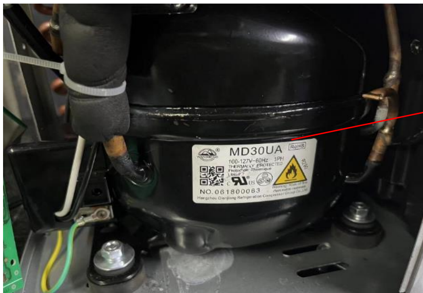
Photo 25 - Compressor MD30UA view
