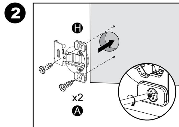
Attach hinges (H) to door with screws (A).
