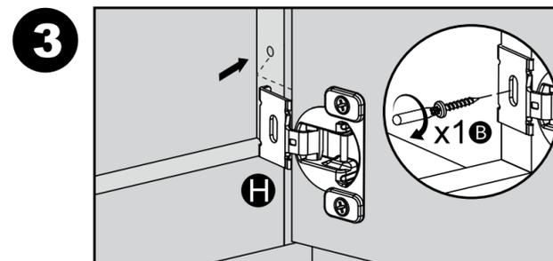
Place door in desired position; mark and drill 3/32" (2.4 mm) pilot holes on frame.
