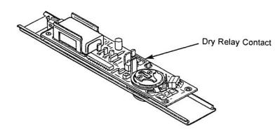
B- Use Dry Relay Contact shown in diagram to connect Alarm Unit to a magnet or strike as desired. For a more audible or visual alarm, a DC hom or light could be used in place of magnet or strike. See step 3 for different wiring diagrams.
