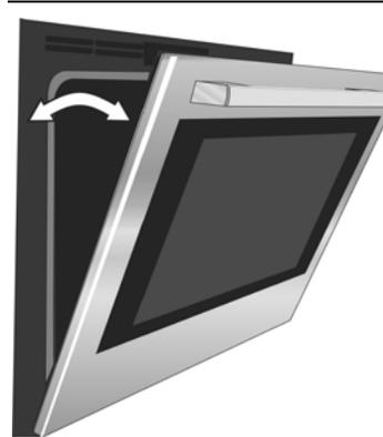
4. Close the oven door until it catches on the hinge stop levers. The door will be open about 7 inches at the top. This takes the spring tension off the hinges so the door can be easily lifted out.
