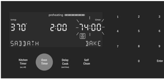
2. Press **Enter** to accept the default 74:00 hours and start Sabbath Mode. Or use the numeric keypad to enter the desired Sabbath mode timer value. Timer values between 0:01 and 74:00 can be entered.
