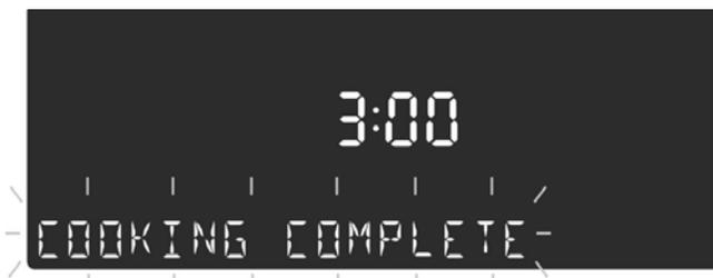
This screen remains in the display until it is cleared by pressing the **Oven Clear/Off** touchpad or until the probe is removed. The display then goes back to stand by mode.
