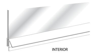
12 Place the sweep onto the bottom of the door. Stand inside the shower, close the door and mark the deflector part of the sweep at the inside edge of the strike jamb.
