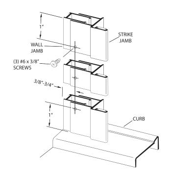
6 Slide the hinge jamb of the door panel assembly over the mounted wall jamb so the door will open outward. Adjust the door panel assembly so there is a 1/4" clearance between the strike jamb and the strike edge of the glass door with it being in the closed position.
