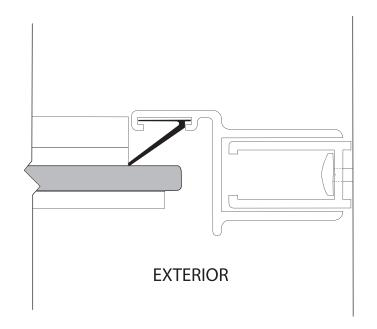
12 Carefully silicone the seam between the walls and the wall jambs as well as the curb and threshold on the inside of the shower.
