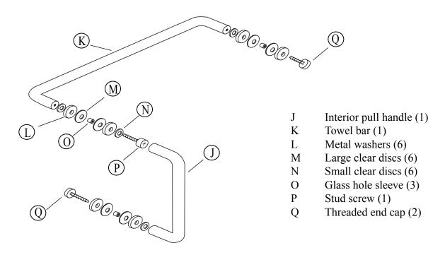
STEP 1 Take the stud head screw and sleeve a 1 1/4" washer on it. Now take both end caps with a threaded stud protruding and sleeve a 1 1/4" washer on them. Sleeve a clear gasket on each of the screws.
