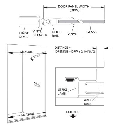
Inside the shower enclosure, using the pencil marks on the wall jambs from the previous step, drill two 1/8" holes through the strike jamb [H] and into the wall jamb 3/8" to 3/4" from the wall and approximately 1" down from the top and up from the bottom of the strike jamb. Drill a third hole centered between the first two
