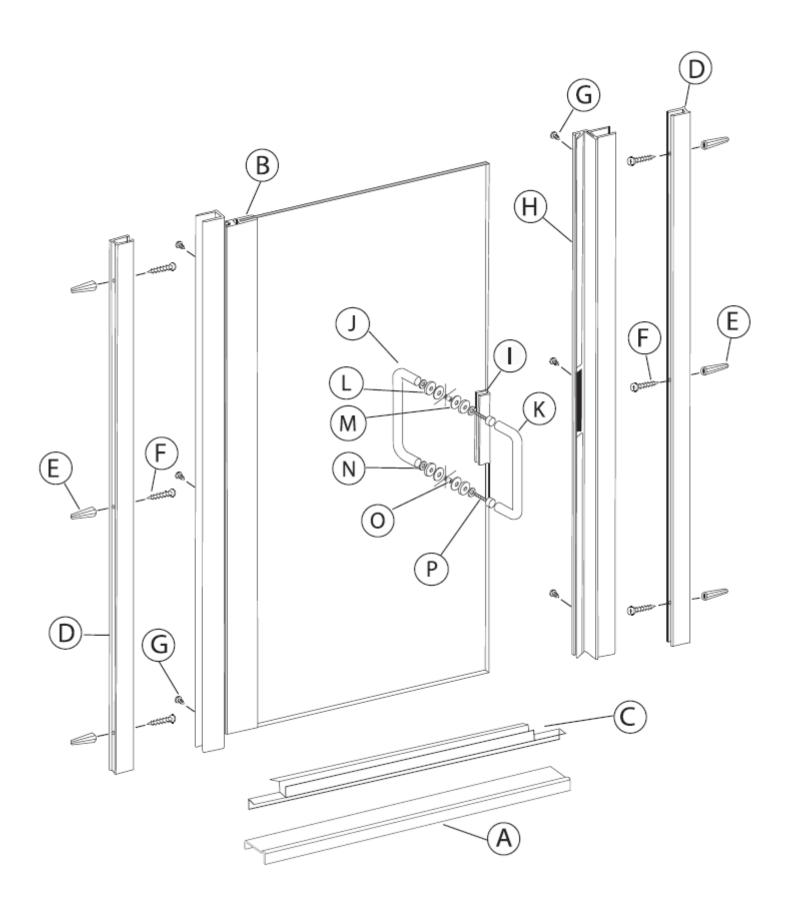
The 1/4" frameless door is completely reversible and may be installed hinge-right or hinge-left. Refer to the illustration to determine the best hinge position for your installation.
