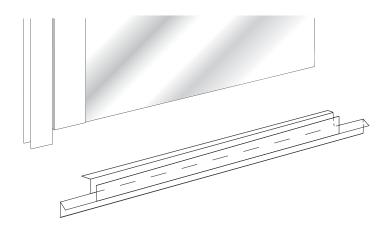
11 Align the clear bottom sweep to the bottom of the door with the deflector lip on the inside of the shower door. Mark the strike side of the bottom sweep even with the strike edge of the door.
