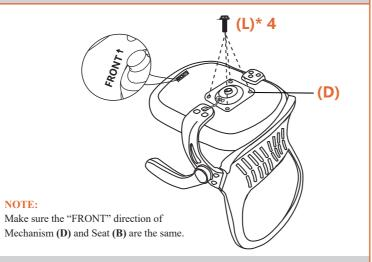
Using Wrench (M), attach Mechanism (D) to the Seat (B) with Bolts (L)\*4.
