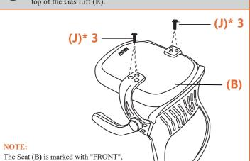
Turn the Seat (B) upside down . Using Wrench (M), install Armrests (C)\*1L\*1R to the Seat with Bolts (J)\*6.
