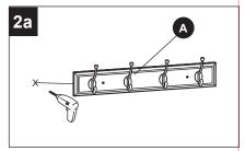
For drywall installations, remove rail (A) and drill 5/16 in. pilot holes at marks. Place anchors (BB) into holes.
