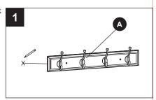
For solid wood/wood stud installations, remove rail
