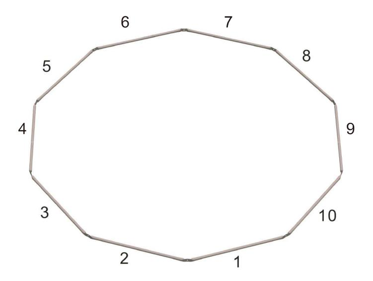
Slide an M8 Washer(#H) over  $\phi$  1 0 x 25mm Bolt(#F), then slide the Bolt(#F) through the joint of 2pcs Coffee Tubes(#A) on the ground, 1pc Blue Tube(#B) and 1pc Coffee Left Gate Tube(#N) in the order indicated by the numbers. Slide another M8 Washer(#H) over the Bolt(#F) and secure with an M8 Nylon Nut(#G).
