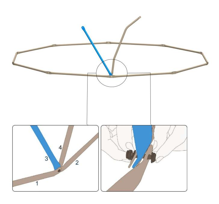
Attach a Blue Tube(#B) and the Coffee Right Gate Tube(#O) to the bottom joint in the right, slide a  $\phi$ 10 x 25mm Bolt(#F) through an M8 Washer(#H), the four tubes (in the same order indicated above), another M8 Washer(#H) and an M8 Nylon Nut(#G).
