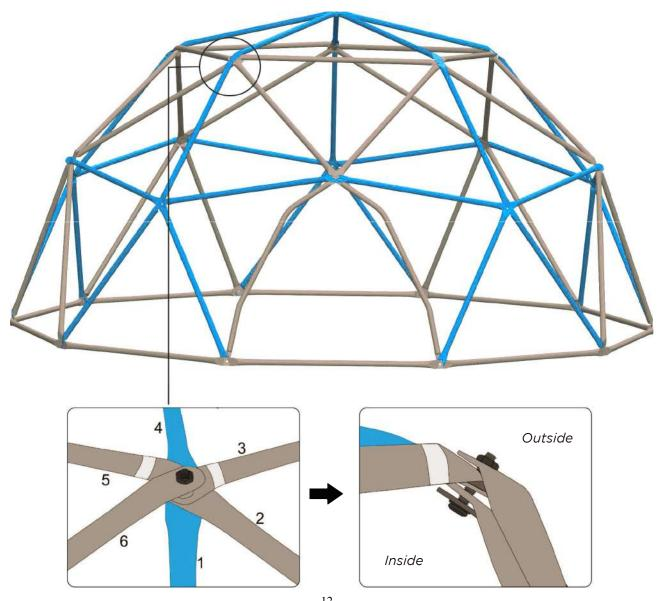
Secure the joint on top with 1pc M8 x 40mm Bolt(#E), 1pc M8 Washer(H) and 1pc M8 Nut(#K).
