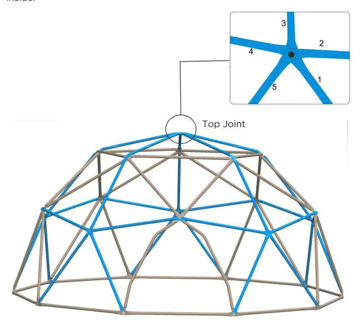
**Step 9**Install the Climbing Grips(#C) with M8 x 25mm Nut(#D) to cover the the bolt on each of the joint (except the bottom joints touching the ground).
