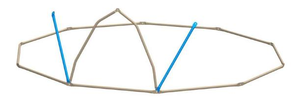
Repeat the same step to attach a Blue Tube(#B) and a Coffee Tube(#A) to the next joint, and secure with 1pc  $\phi$ 10 x 25mm Bolt(#F), 2 pcs M8 Washer(#H) and 1pc M8 Nylon Nut(#G).
