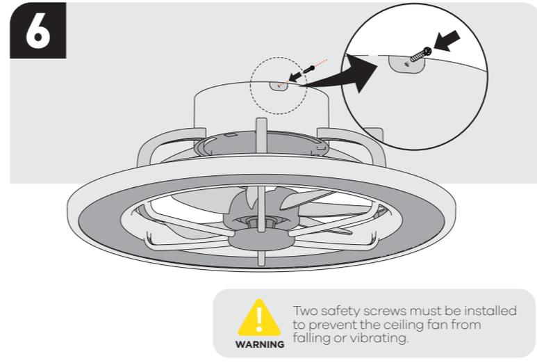
**WARNING** ! Two safety screws must be installed to prevent the ceiling fan from falling or vibrating.
