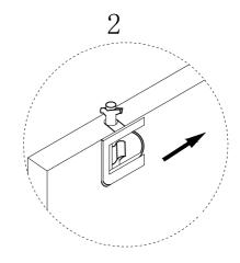
Align the cross shape of fastener B'' on the vertical plate with the hole position on the top plate and bottom plate,
