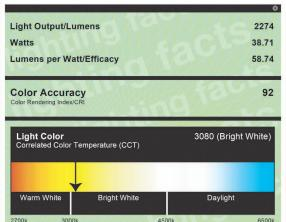
All results are independently verified according to IES LM-79-2008: "Approved Method for the Electrical and Photometric Testing of Solid-State Lighting."
