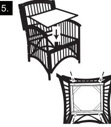
STEP 4 : PUT SEATING FRAME DOWN ON THE CHAIR. FIX THE SEAT BASE WITH WOODEN SCREW 40 MM FROM THE BOTTOM ON EACH 4 CORNER.
