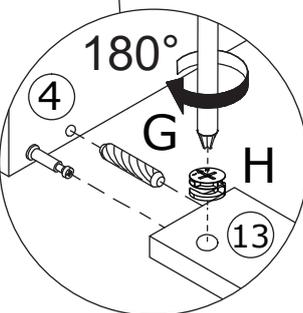
Connect board 4 and 5 to board 12, 13 and 9 using wooden dowel(G), add cam lock(H) into board 12, 13, 9 and turn clockwise to tighten as shown.
