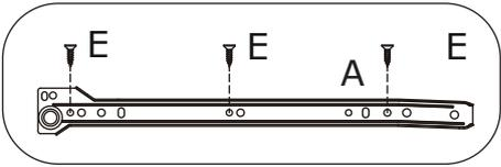
Fix rail(A) to board 4 with screw(E) as shown.
