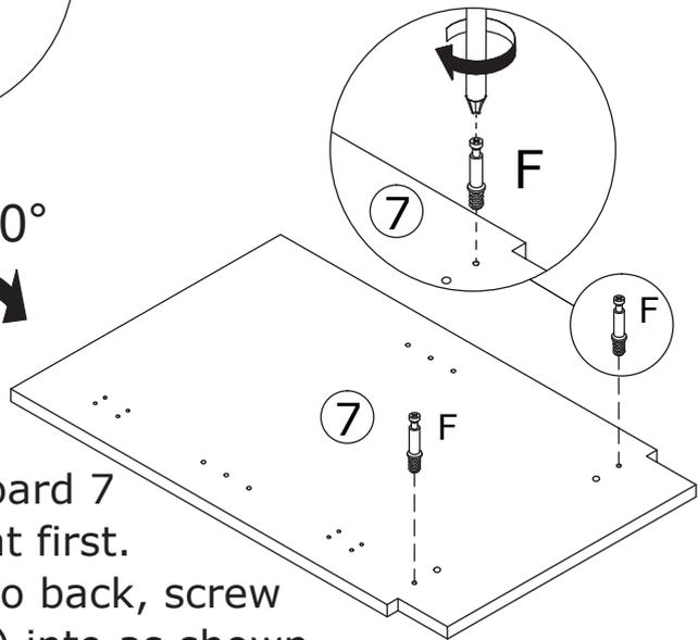
Fix rail(B) to board 7 with screw(E) at first. Flip the board to back, screw eccentric rod(F) into as shown.
