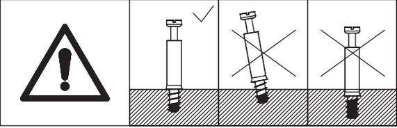
Screw eccentric rod(F) into board 21 as shown.
