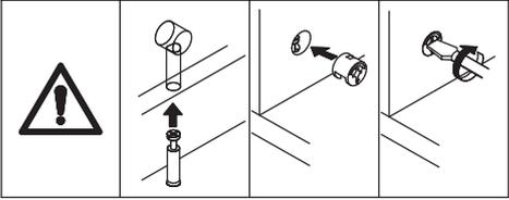
Attach board 21 to board 22 and 23, add cam lock(H) into and turn clockwise to tighten as shown.
