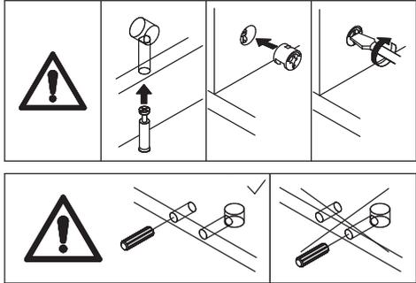
Connect the two assembled components using wooden dowel(G), add cam lock(H) into and turn clockwise to tighten as shown.
