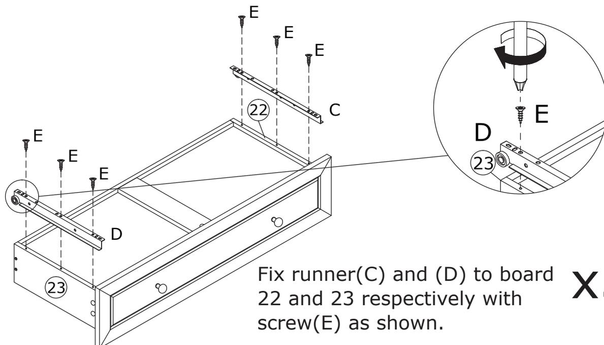
Fix runner(C) and (D) to board 22 and 23 respectively with screw(E) as shown.
