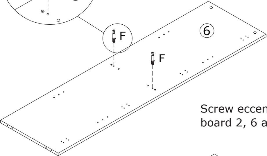
Screw eccentric rod(F) into board 2, 6 and 3 as shown.
