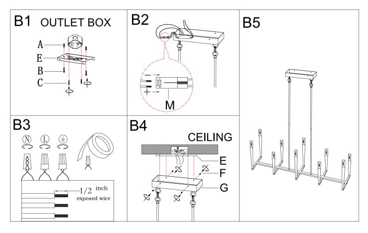
Step B1 » Carefully pass the supply wires from the outlet box through mounting plate (E).
