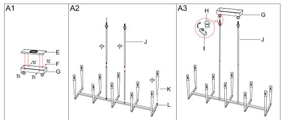
Step A1 » Unscrew canopy screws (F) from mounting plate (E) and canopy (G).
