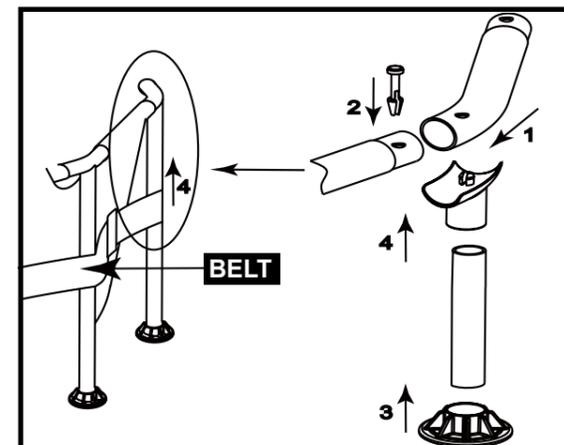
1. Use the connection end of the T-Joint to connect the adjacent horizontal tubes.
