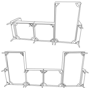
STEP 5: Assemble the Back frame (J) with Bolts (O) and Washers(N).
