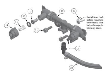
Insert Boom Hose Assy. (22) in boom and secure with Quick Clip (13)
