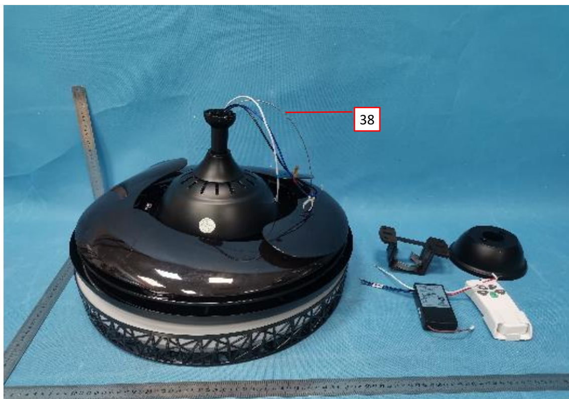
Photo 14 - Contruction with additional steel rope support of all models for cETLus and cETL
