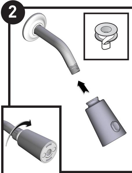
Wrap shower arm with thread seal tape. Thread showerhead onto shower arm.
