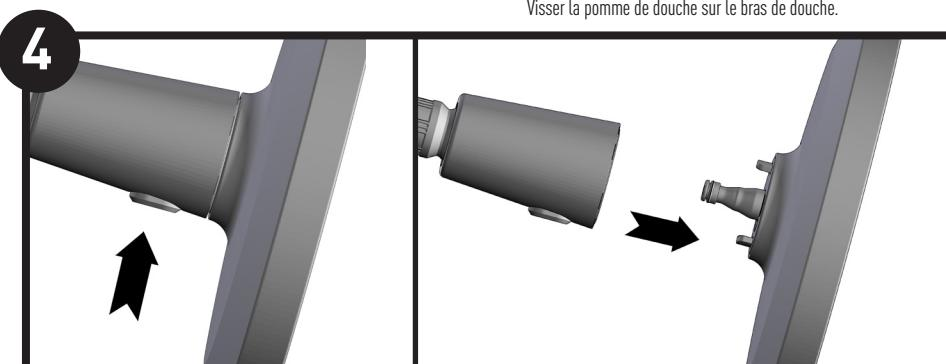
To remove showerhead for easier cleaning press the button on the docking bracket and pull the showerhead away from the docking bracket.
