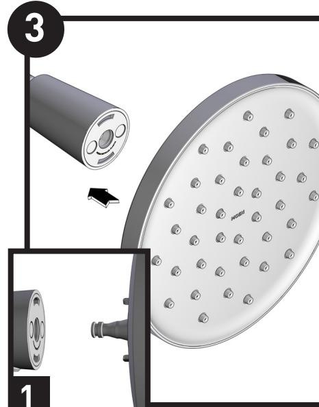
1. Align tabs on showerhead with mating feature in docking bracket.
