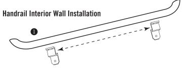
1. On the ground, layout handrail and wall brackets to ensure you will achieve your desired look and symmetry once the handrail is installed.
