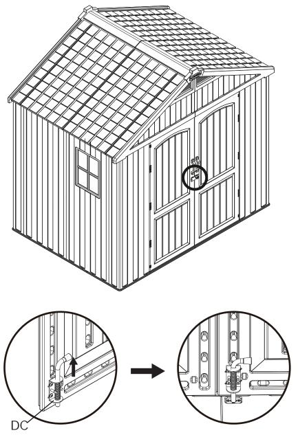
Remember to unplug the DC when closing the door and put it down when the door is closed.
