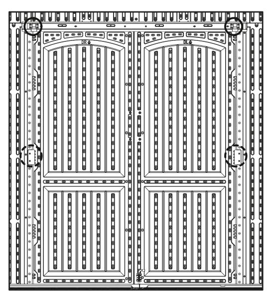
Two people are needed. One person closes the door and inserts the pin, while the other person adjusts the gap outside the door. After making sure the gap is even, the person inside installs DDZ screws SP6-20.
