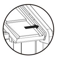
D1 and D3 are placed in the grooves of the iron frame, aligned with the grooves of the CL CR respectively and pushed forward.
