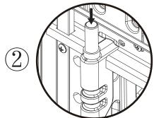
Push it into the groove of the floor. Press the DZ downwards.
