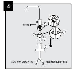
Attach the mixer (1) to the standpipe (2), make sure the prongs (3) on the standpipe (2) insert into the hole (4) of the mixer (1). Install the set screw (5) and tighten into the standpipe (2) with hex wrench. Note: Do not to reverse the cold and hot supply lines.
