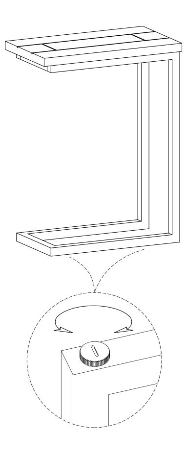
**Note**: Levelers on bottom of legs can be adjusted if floor is uneven.
