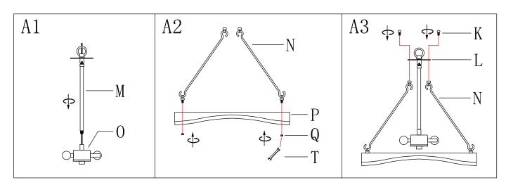
Step A1 » Screw pipe (M) onto sockets assembly (O).
