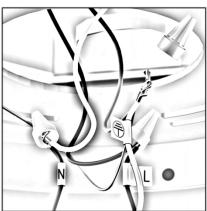
2) Use the provided screws (B) to secure the mounting bracket (A) to the junction box.
