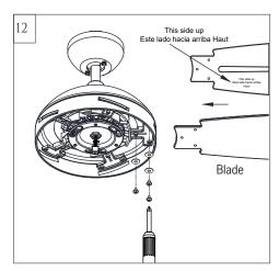
Insert blade into the slot on flywheel. Install blade with screws and washers provided, aligning each of the holes as shown and tighten all screws securely. Repeat this process for remaining blades.
