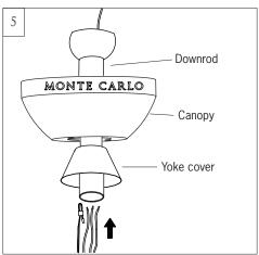
Place downrod over canopy and yoke cover. Thread lead wires and safety cable from motor assembly through downrod.
