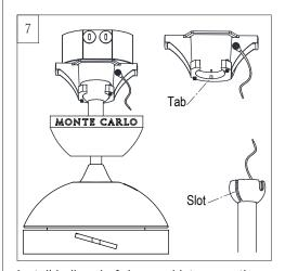
Install ball end of downrod into mounting bracket opening. Align (engage) slot on ball with tab on mounting bracket. **Warning:** Failure to align slot on ball with tab may result in serious injury. **Important:** If using the angle mount,
