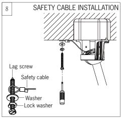
For Canadian installation and for USA fan and light kit combinations over 35 lbs, in both flush and downrod modes the safety cable must be installed into the house structure beams using 3" lag screws, washers and lock washers provided. Make sure that when the safety cable is fully extended the lead wires are longer than the cable and no stress is placed on the lead wires.
