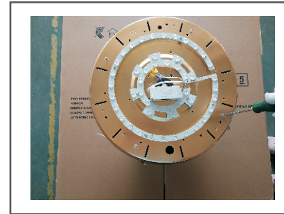
Step 4. Remove the main engine chassis screws.
