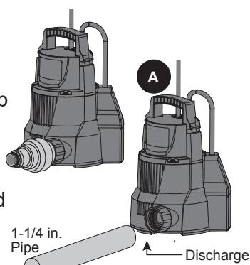
1. Install the snap-on strainer (C) by lining up the pump (A) base to match the strainer. Push down gently until it latches.
