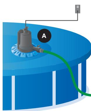
5. Plug the pump into a properly grounded, GFCI 115 V outlet. For safety, the pump should always be electrically grounded to a suitable electrical ground, such as a grounded water pipe, properly grounded metallic raceway, or ground wire.
