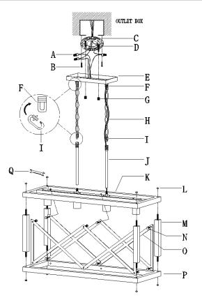
Step A1: Pass the batten (M) through the lower wooden frame (P) and secure with a hex nut (L). Pass the batten (M) through the upper wooden frame (K) and secure with a hex nut (L).
