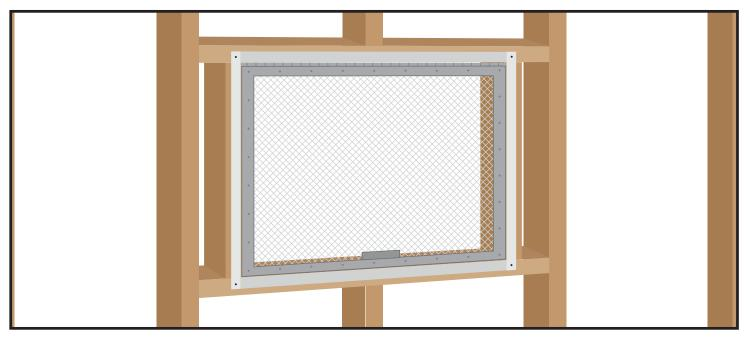
24 in. x 18 in.is the minimum size for a building code approved crawl space access. 36 in. x 24 in. is the minimum access for a crawl space access with mechanical equipment.
