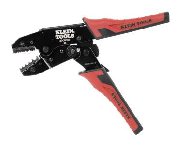
The full-cycle Ratcheting Crimper crimps 10-22 AWG non-insulated wire terminals. This tool features five crimping cavities in one tool for five size ranges of non-insulated terminals. Crimper design provides low effort to crimp while maintaining a high terminal pull-off force. Built-in ratchet ensures full-cycle crimping for a uniform crimp every time. Compound lever-action of narrow-span handles puts more crimping power into each squeeze. Comfort grips help reduce hand fatigue.
