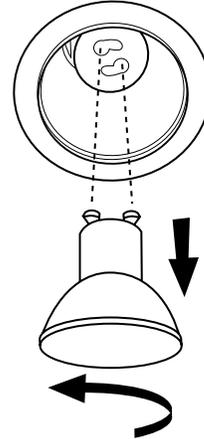
3. Remove the bulb and replace it with a 120-volt, 6.5-watt maximum LED bulb with a GU10 base. Turn it clockwise to lock it into place.
