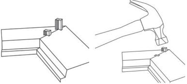
Holding the two corner pieces level and in place, insert both assembly wedges into the correct route. Insert the pointed end first. Tap the frame wedges flush with the back of the frame. Repeat for all corners.
