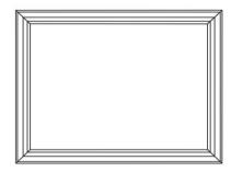
Turn over and inspect all corners. Wipe off excess glue with a damp cloth. Before the glue dries, if necessary, adjust the corners. One frame side may be higher than the other.
