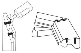
Choose a corner and apply glue to both pieces. With both glued pieces face down, level and align the corner and the routes. Depending on the profile, a door stop may be needed to level the frame.
