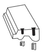
Match the length of assembly wedges to the depth of the routes.
