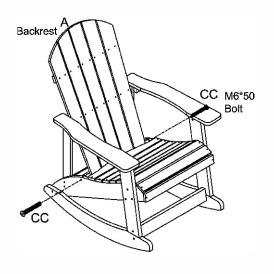
**STEP 7B:** Attach the rear of the Left Armrest (Part C) and Right Armrest (Part D) to the Back Supports (Part E) and Backrest (Part A) using (2) M6\*70 Bolts (Part EE).
