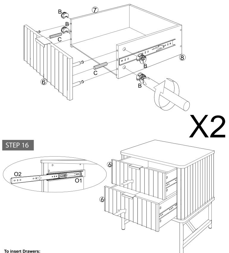
a) Bring the ball-bearing slider on Drawer Glide Track(O1) forward to the front edge of(O1). b) Align the back open-end of the Drawer Glide Runner(O2) on each side of the drawer to fit squarely into the groove on the open front-end of(O1).Be sure the drawer/O2 is not tilted or angled, and gently push in drawer squarely.
