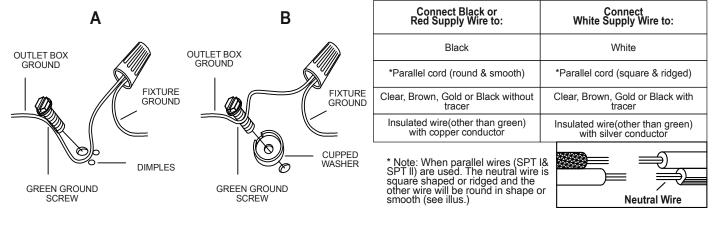
• Twist wires together with plastic wire connectors (A) until tightly joined.
