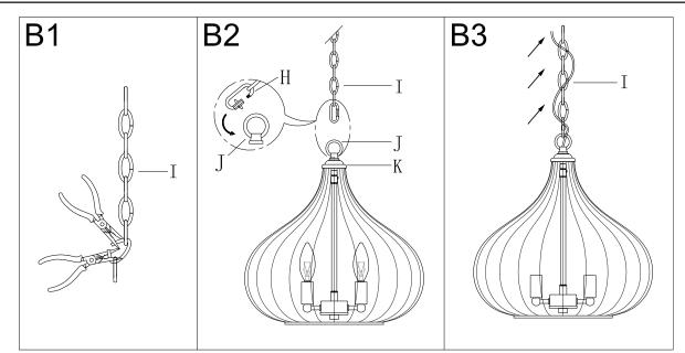
Step B1 » By measuring, determine the correct number of links needed for proper hanging height. Using the chain pliers, disconnect and discard the unwanted part.
