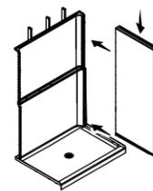
**12** Push the end wall into the back wall to compress the seam and flex the lower back wall into the vertical position.
