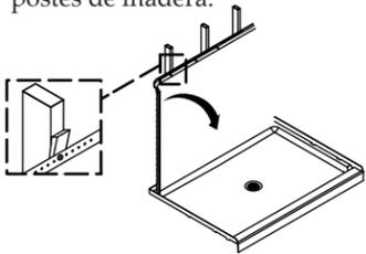
**5** Secure the flange to the studs.
