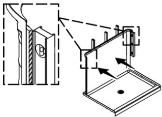
**4** Add 1/8" (3 mm) additional shim behind top flange of lower back wall, tipping the wall into the stud pocket.
