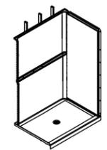
**13** The front edges should be flush, with no more than a 1/32" (1 mm) gap.
