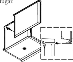
**7** Temporarily secure the upper back wall with one screw in the center of the flange.
