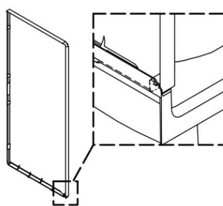
**11** Fit the end wall flanges into the back wall channels as shown. Push the end walls forward and down.
