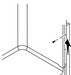
**15** Remove the temporary screw from the upper back wall. Shim if necessary and secure the flanges to the studs.
