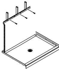
**6** With the upper wall tab engaged with the lower wall slot, push the upper wall into place.
