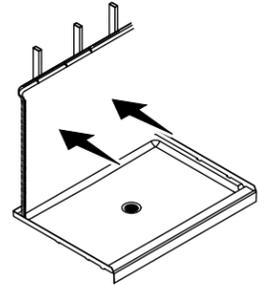
**3** Plumb the lower back wall on the hatched surface as shown. Use the provided shims if necessary.
