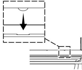
**2** Push the top and bottom of the lower back wall toward the studs.
