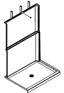
**8** Measure, mark, and drill the faucet holes in the end wall.
