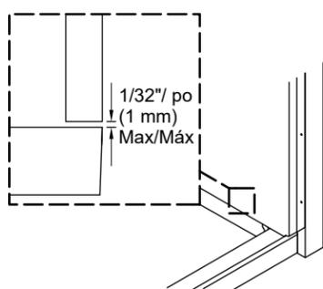
**14** Starting at the bottom of the wall, secure the wall flanges to the studs with screws.
