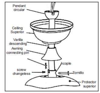
Remove connecting pin and unscrew it. Lead cable in through the lowering lever, considering these parts.
