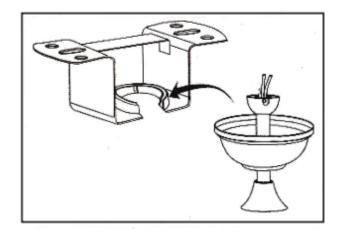
2.Carefully lift the fan joint and place it on the shaft of the hanger. Make sure that the hole of the bracket and the structure to be connected are aligned with the upper flange of the hanger. After wiring, press upward and twist to adjust the position of the screw hole to connect the canopy to the suspension bracket. Later, Connection of fixing screws.
