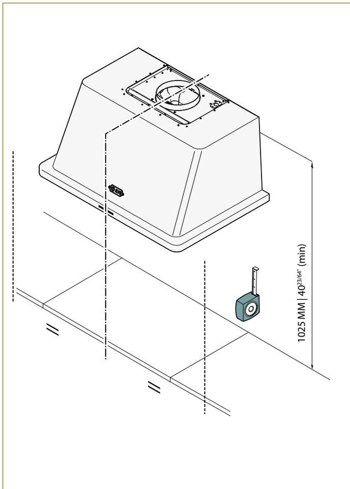
The fastening kit (screws and plugs) supplied with the hood can only be used on masonry wall. For installation on other types of walls consider alternative fastening systems, taking into account the strength of the wall itself and the weight of the hood.
