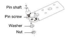
9. Install the lower hinge on the left side of the cabinet.
