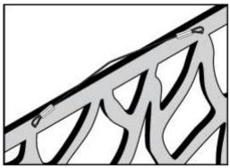
• Using a wire rope or string. Mark the centre of the panel on the back using a tape measure, then mark screw positions equal distance from the centre. Secure the wire rope or string to the panel by using short screws up to 1/4" long.
